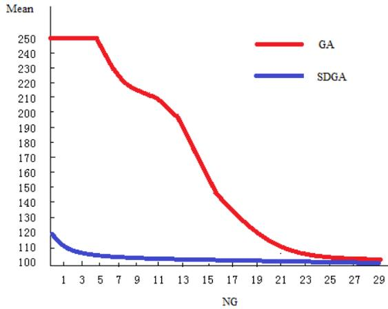
Fig. 2. Change of cost average in a 15 node example
